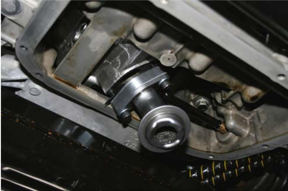
The first step is to clean all the gasket compound of the face of the existing engine casting to give a nice smooth surface. Use a flat blade for this but do not gouge or mark the surface. Be gentle and patient; Once this surface is nice and clean place the pickup and extension into position. Let it hang there, do not tighten it yet 😊
