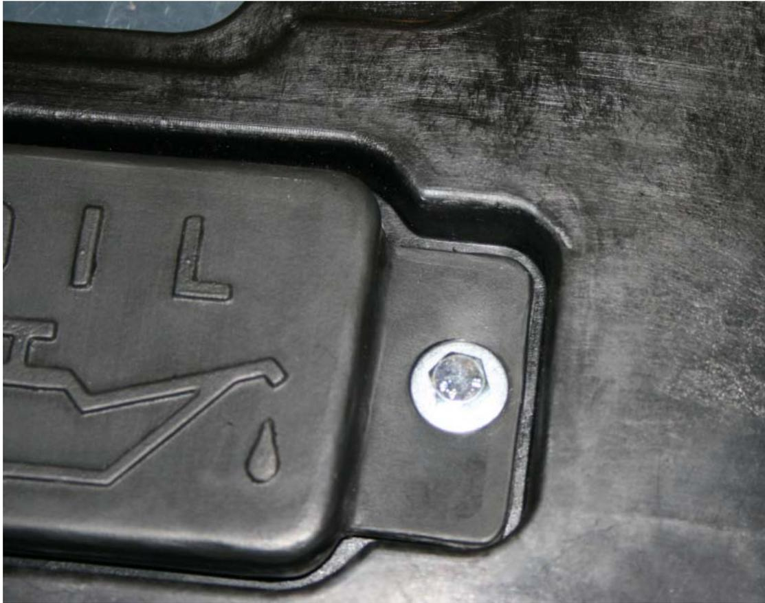
The new shorter bolt and washer assembly can now be fitted to the oil cover hatch as pictured. This is important to stop any contact between the factory bolt and the pan cover.
