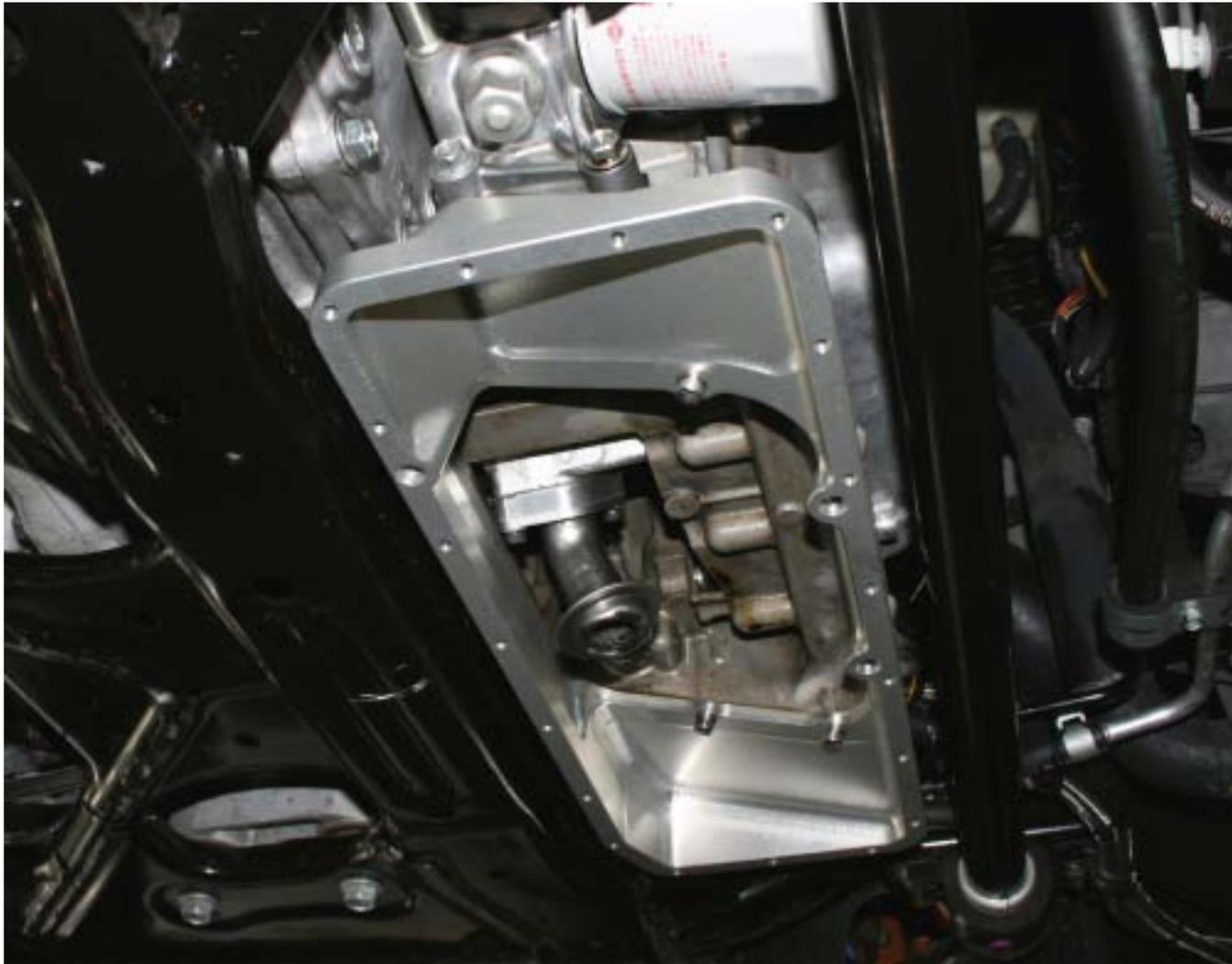
Its now time to fit the main WR35OP body to the bottom of the factory casting. Use the stainless cap screws and locking washers for this. Once the body is fastened into position the oil pickup can now be finally tightened and left in place. Note, there is no sealant used in any part of this installation. Its totally 'dry' thanks to the use of O-rings! Getting at the rear bolts requires the use of a ball headed Allen key.
