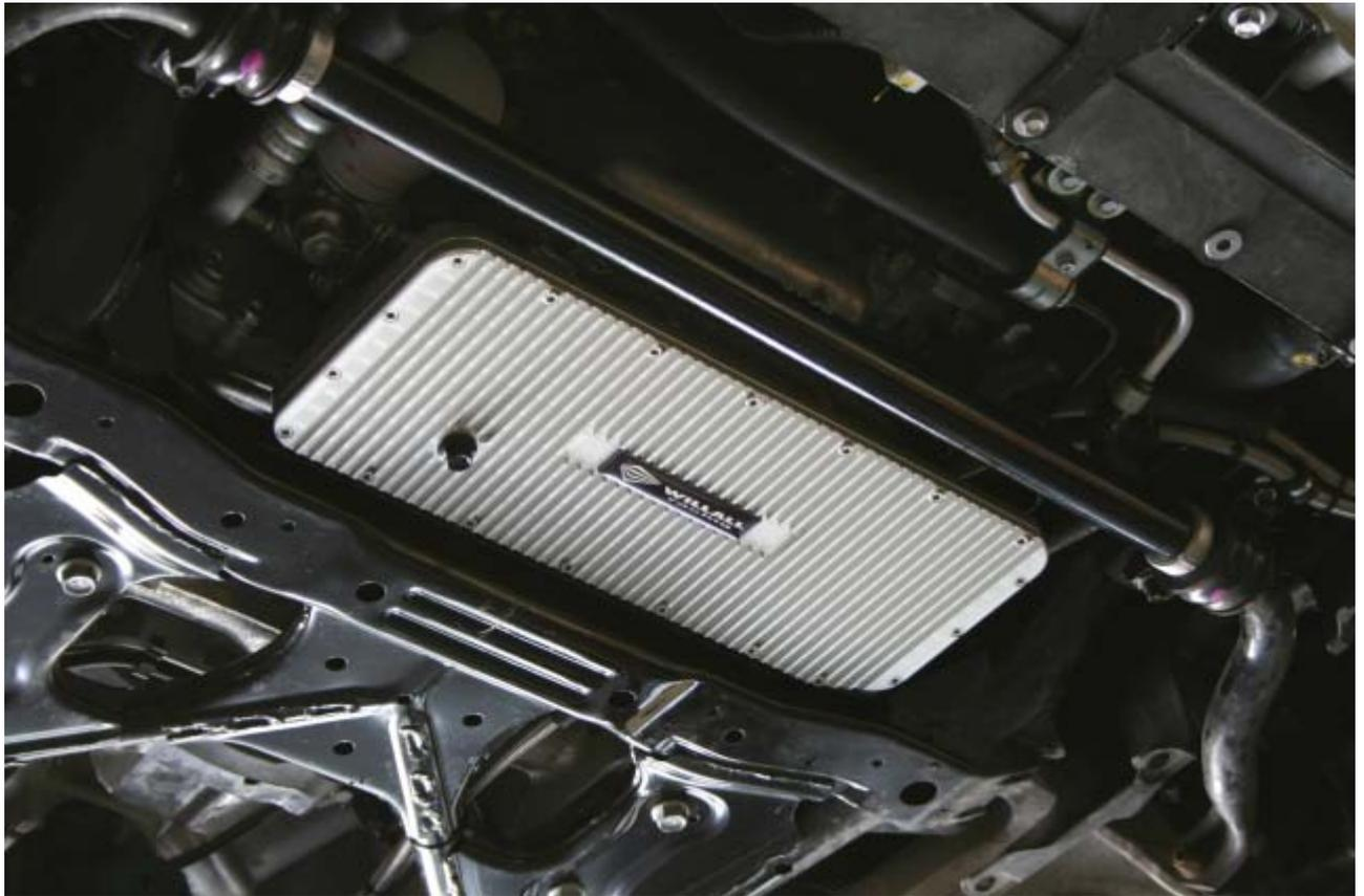
The finned WR35OP pan cover now pushes up against the bottom of the main body and screws into position. Once more the O-ring in the plate provides all of the sealing required. The factory Sump Plug then screws directly into the WR35OP and locates exactly over the top of the factory oil hatch.
